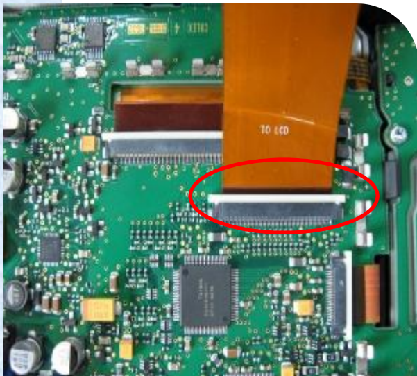
Connect the other side of FPC cable to the connector from LCD.
