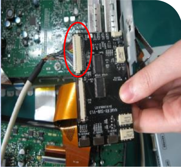
Connect LCD cable from Interface to sub-board.
