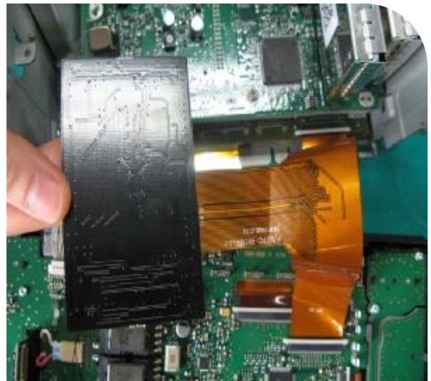
Connect FPC cable to sub-board.
