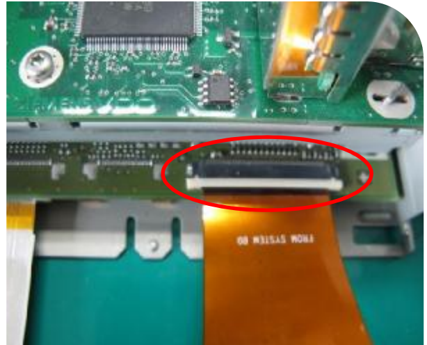
Connect FPC cable to the indicated connector from System Board of HU.
